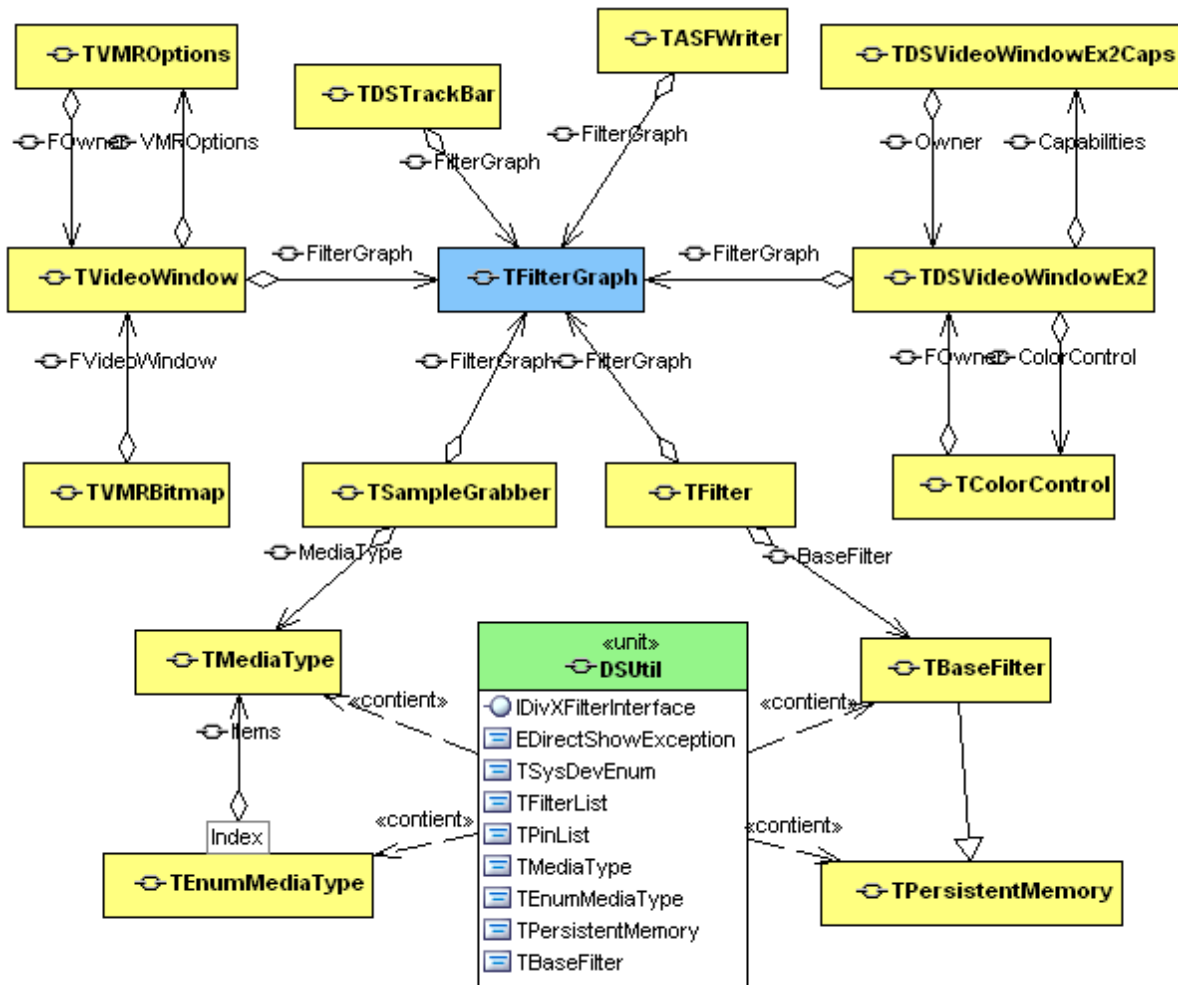
Fig. 1. Structure of DSPack
